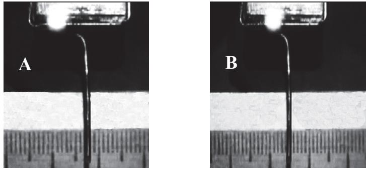
**FIGURE 2.** Frames of high speed velocity photography of pendulum deflection. A:  $n = 0$ ; B:  $n = 43$  ( $n$  – number of frame)
