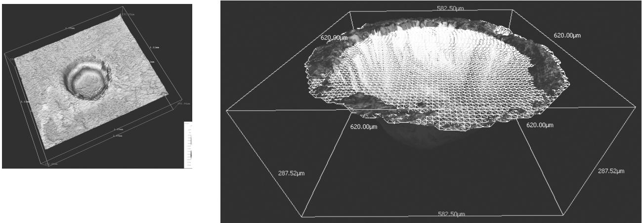
**FIGURE 4.** 3D image of crater. Laser energy is equal to 9.4 J
