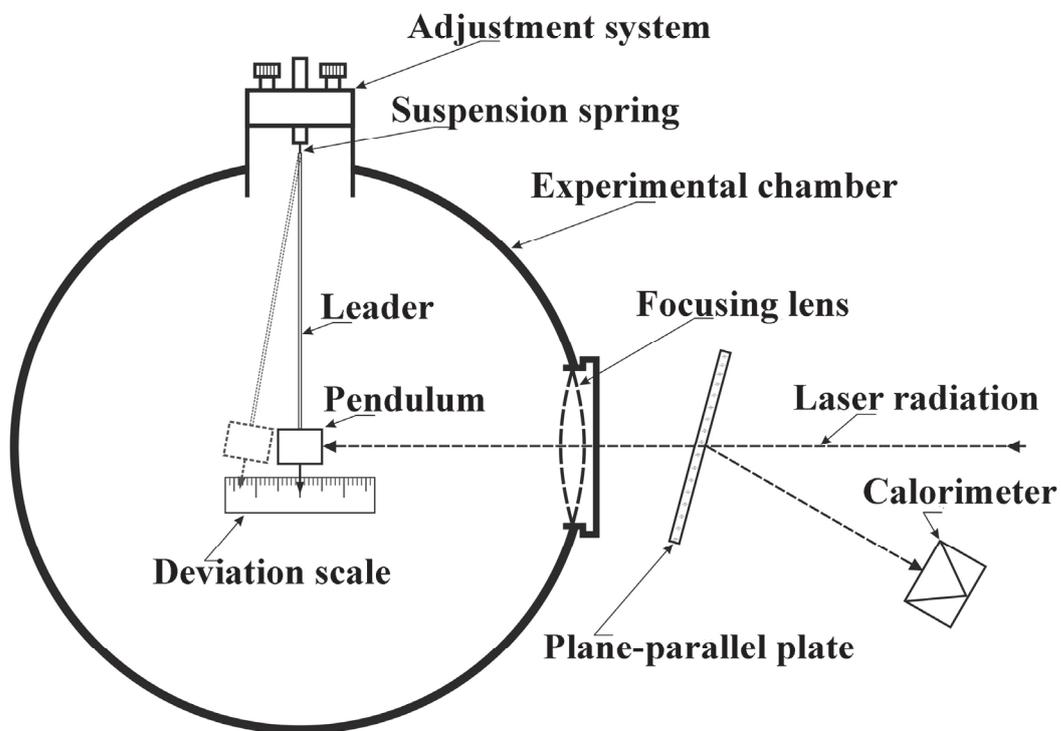
**FIGURE 1.** Scheme of experiment
