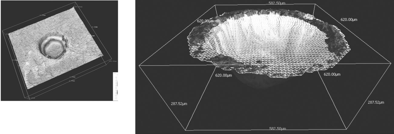
**FIGURE 4.** 3D image of crater. Laser energy is equal to 9.4 J
