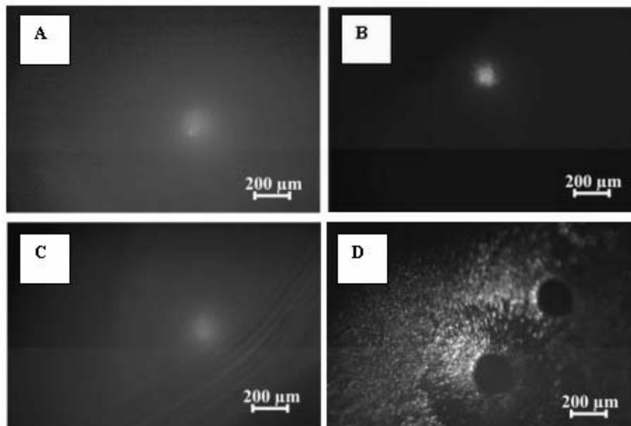
**Figure 7.** Images of laser plasma in  $(3/2)\omega_0$  (C),  $2\omega_0$  (D), and  $(5/2)\omega_0$  (B) radiation, correspondingly ((A) – craters in Cu target, density power of heating laser radiation  $\sim 2 \cdot 10^{14} \text{ W/cm}^2$ ,  $T_e \sim 300 \text{ eV}$ ).
