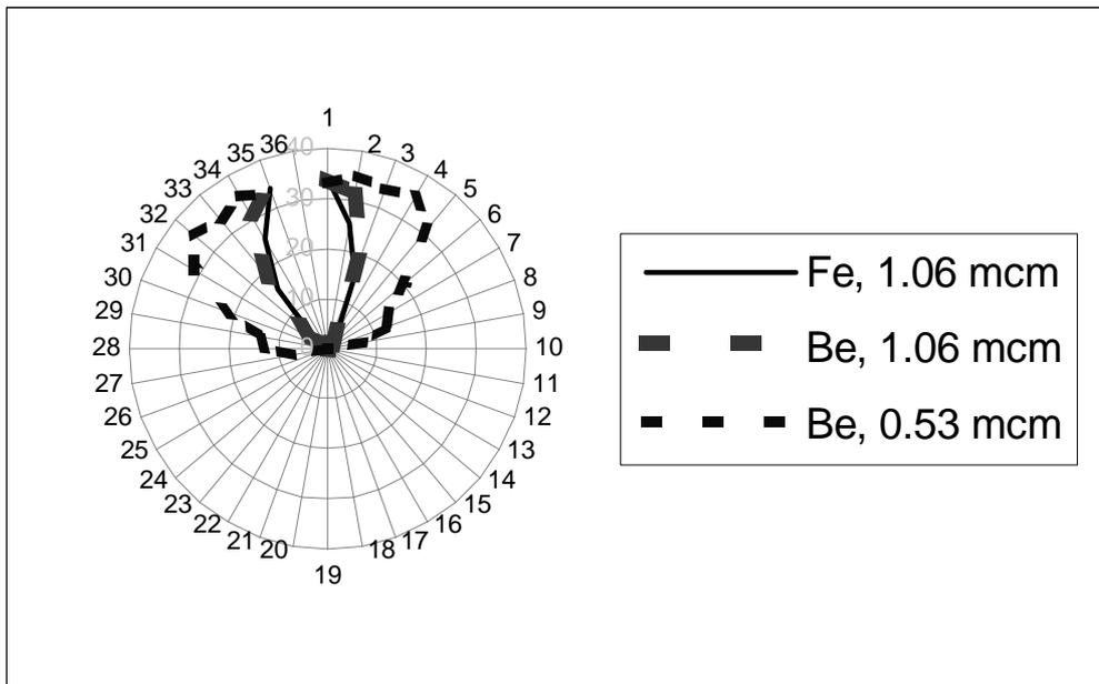
**Figure 5.** Angular distribution of radiation scattered at the fundamental frequency (1.06 μm) and the second harmonic frequency (0.53 μm).
