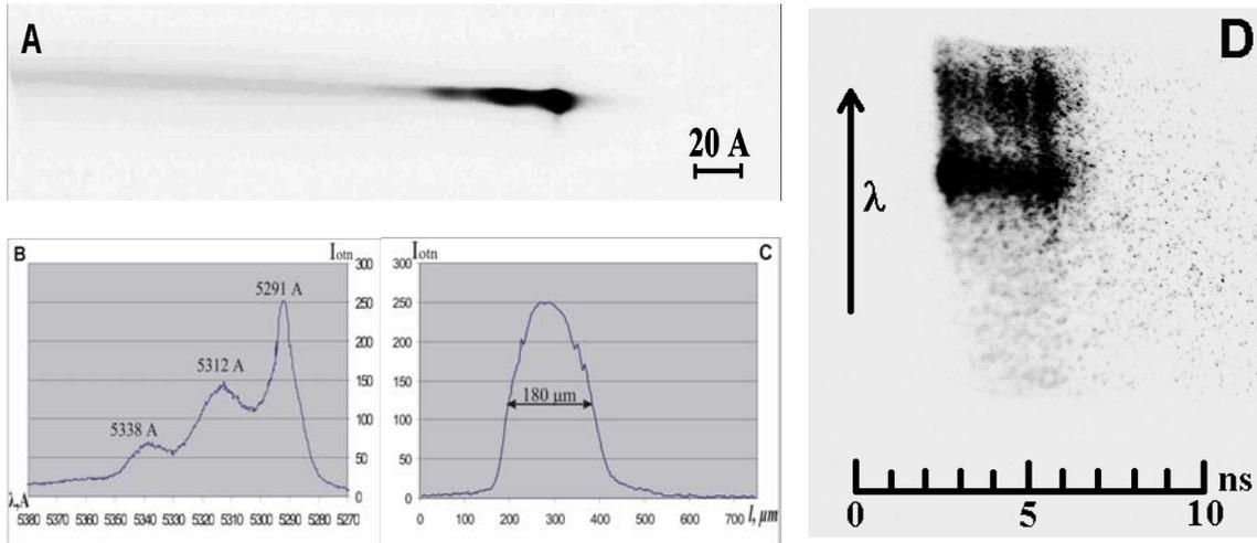
**Figure 8.** The second harmonic generation. A – spectrum of  $2\omega_0$ , B – spectral distribution, C – spatial distribution, D – time-resolved spectrum of  $2\omega_0$ .
