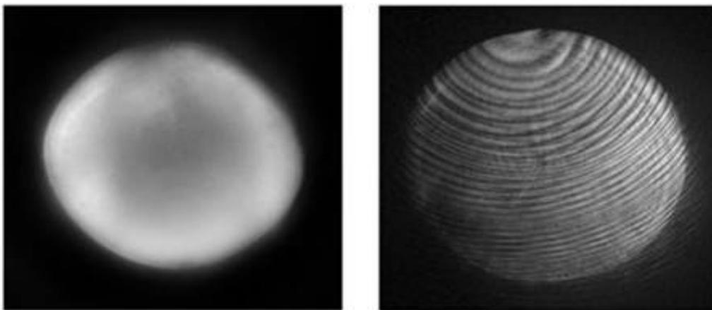
**Figure 2.** Laser intensity distribution (left – radiation of CCR laser, right – radiation of single-mode YAG laser).
