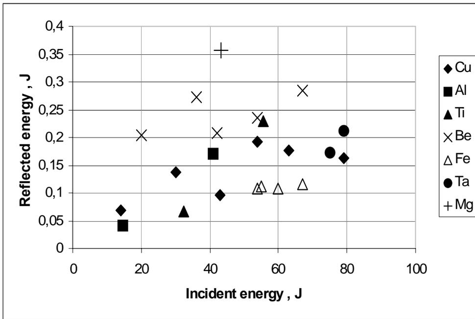
**Figure 4.** Dependence of energy reflected into aperture of focusing lens on the incident laser energy.
