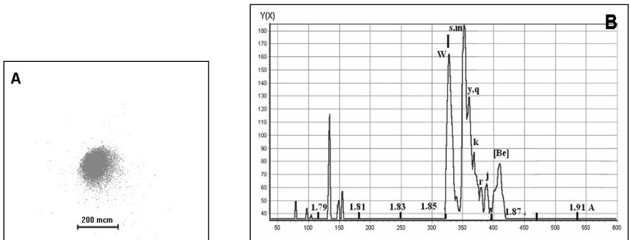
**Figure 6.** A - Image of laser plasma in X-ray radiation received by means of pinhole camera with apertures 14  $\mu\text{m}$ . B - X-ray spectrum of laser plasma radiation from Fe target. Density power of heating laser radiation  $\sim 2 \cdot 10^{14} \text{ W/cm}^2$ ,  $T_e \sim 300 \text{ eV}$ .
