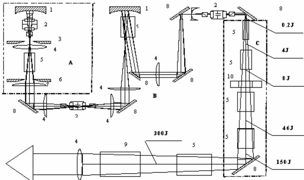
**Figure 1.** Optical scheme of the master oscillator (A), of the system of formation of spatial-temporal characteristics of laser radiation (B), and of the amplify system (C):
